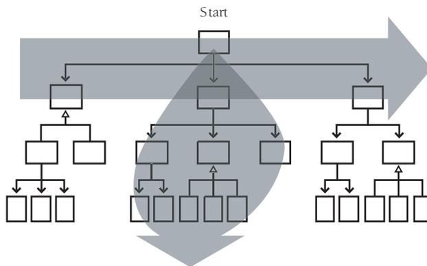
**Figure 29-12** In T-shaped integration, you build and integrate a deep slice of the system to verify architectural assumptions, and then you build and integrate the breadth of the system to provide a framework for developing the remaining functionality.
