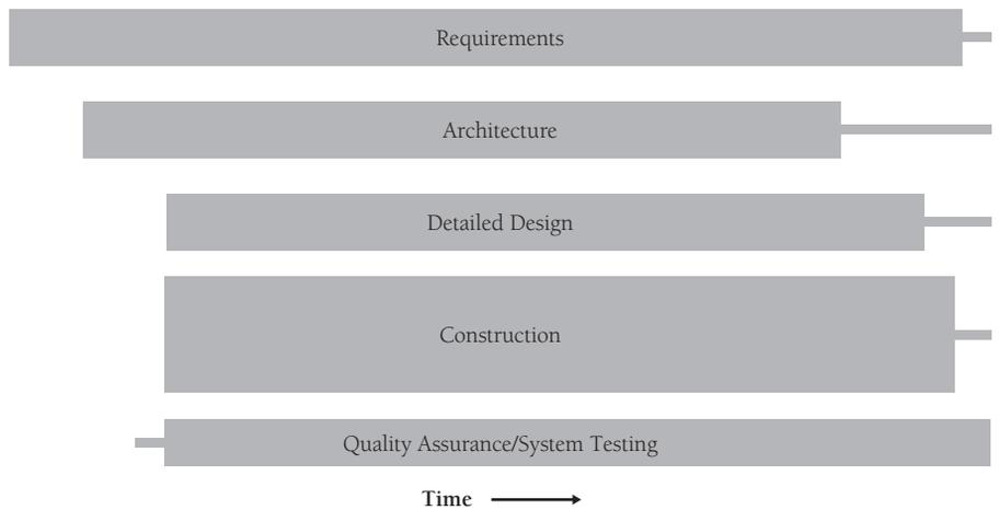
**Figure 3-3** On other projects, activities will overlap for the duration of the project. One key to successful construction is understanding the degree to which prerequisites have been completed and adjusting your approach accordingly.
