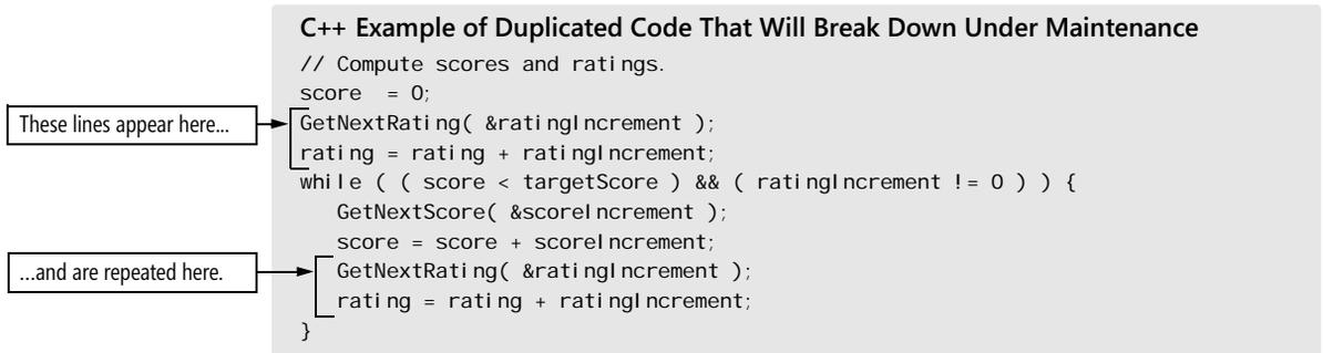
The two lines of code at the top of the example are repeated in the last two lines of code of the *while* loop. During modification, you can easily forget to keep the two sets of lines parallel. Another programmer modifying the code probably won't even realize that the two sets of lines are supposed to be modified in parallel. Either way, the result will be errors arising from incomplete modifications. Here's how you can rewrite the code more clearly:
