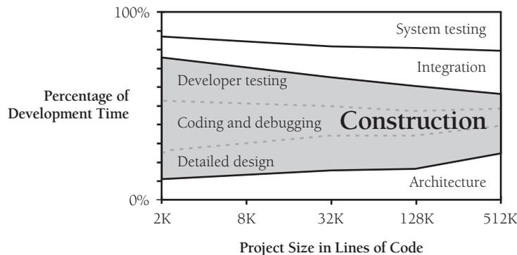
**Figure 27-3** Construction activities dominate small projects. Larger projects require more architecture, integration work, and system testing to succeed. Requirements work is not shown on this diagram because requirements effort is not as directly a function of program size as other activities are (Albrecht 1979; Glass 1982; Boehm, Gray, and Seewaldt 1984; Boddie 1987; Card 1987; McGarry, Waligora, and McDermott 1989; Brooks 1995; Jones 1998; Jones 2000; Boehm et al. 2000).
