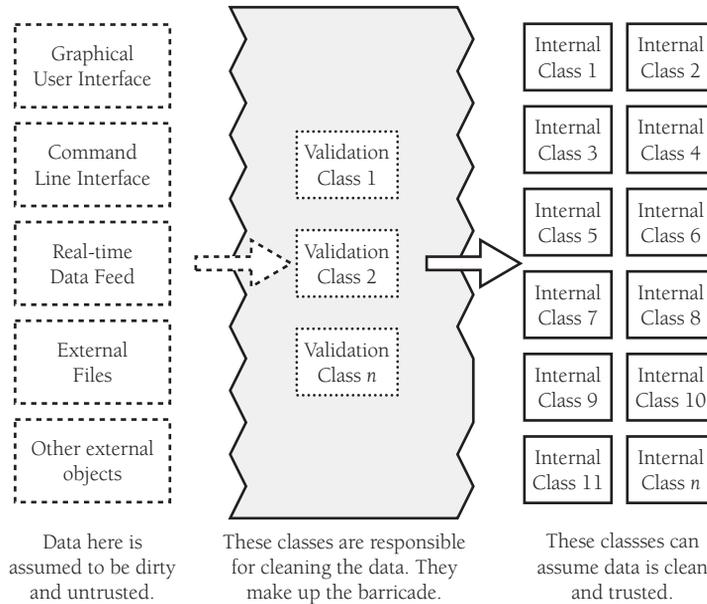
**Figure 8-2** Defining some parts of the software that work with dirty data and some that work with clean data can be an effective way to relieve the majority of the code of the responsibility for checking for bad data.
