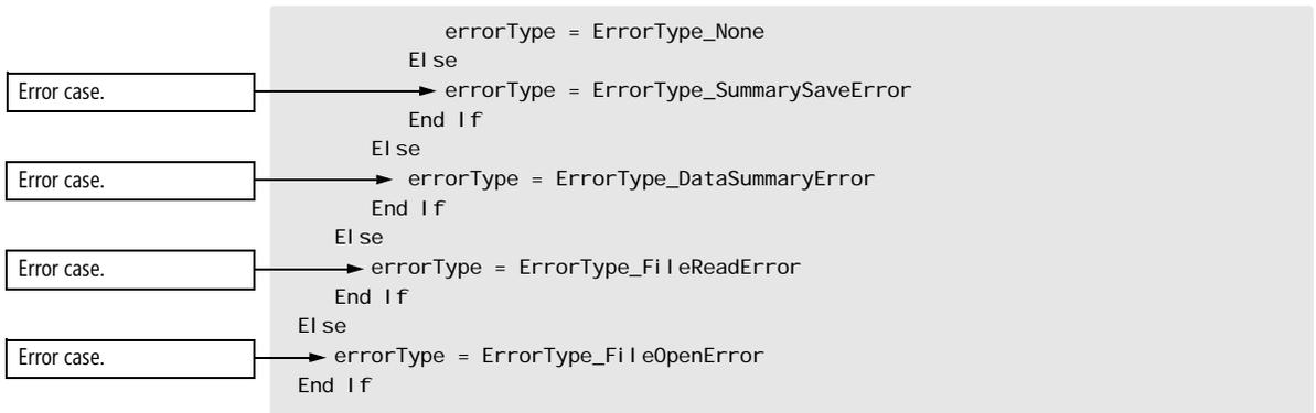
In the revised example, you can read the main flow of the *if* tests to find the normal case. The revision puts the focus on reading the main flow rather than on wading through the exceptional cases, so the code is easier to read overall. The stack of error conditions at the bottom of the nest is a sign of well-written error-processing code.
