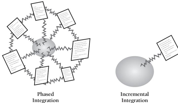
**Figure 29-4** In phased integration, you integrate so many components at once that it's hard to know where the error is. It might be in any of the components or in any of their connections. In incremental integration, the error is usually either in the new component or in the connection between the new component and the system.
