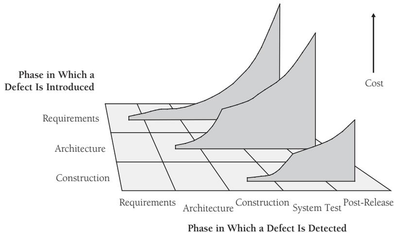
**Figure 3-1** The cost to fix a defect rises dramatically as the time from when it's introduced to when it's detected increases. This remains true whether the project is highly sequential (doing 100 percent of requirements and design up front) or highly iterative (doing 5 percent of requirements and design up front).
